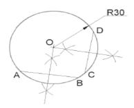
3. Hint : Join 3 points A,B,C which are not in a straight line ,bisect the lines and with the centre O, draw the circle.
